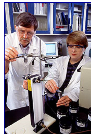
Chemists Wayne Marshall and Lynda Wartelle air-sample volatile organic compounds to determine the adsorptive properties of nutshell carbons. (K8326-5)
