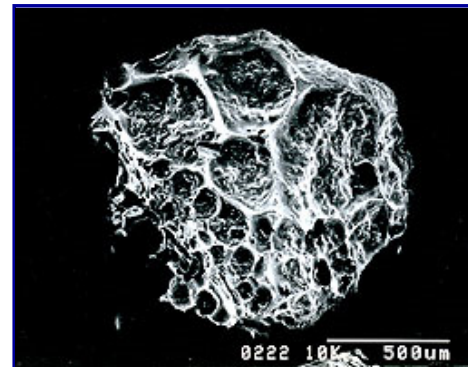
Scanning electron micrograph shows the effect activation has on the gross structure of nutshell carbon granules. While it is impossible to see active micro- and meso-pores, the large pits are significant evidence of gasification.
