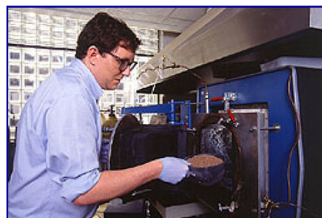
Raw macadamia nut shells placed in a special oven by chemist Chris Toles will be carbonized and activated at temperatures above 800 °C.
