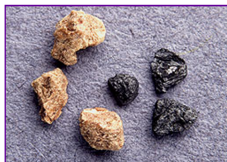
Macadamia shell pieces before and after carbonization.
